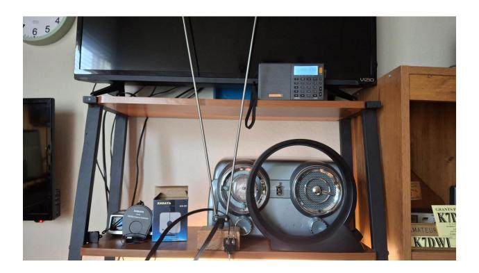
Notice in the picture that the feedline is 300 Ohm Twinline connected to a Balun (300 to 75 Ohm) to a 1/8 inch phono connector for the External Antenna Port..
